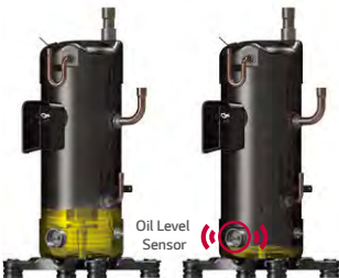
Eliminated Unnecessary Oil Return via Oil Sensor
