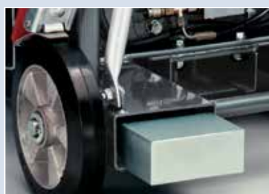
Ballast weights for use with shorter outriggers
