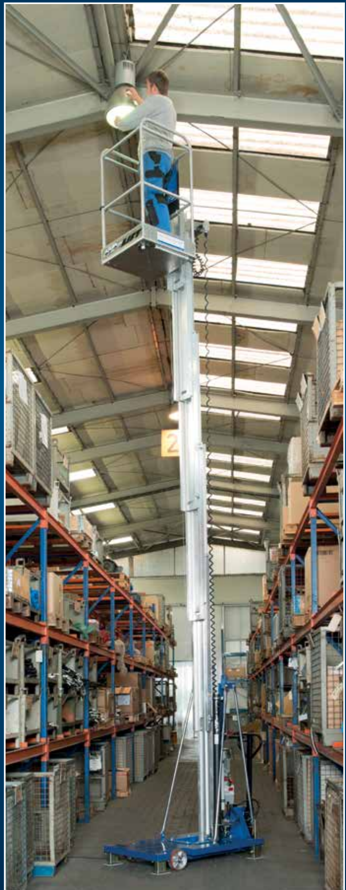
Industrial lifts without outriggers for the use in narrow halls
