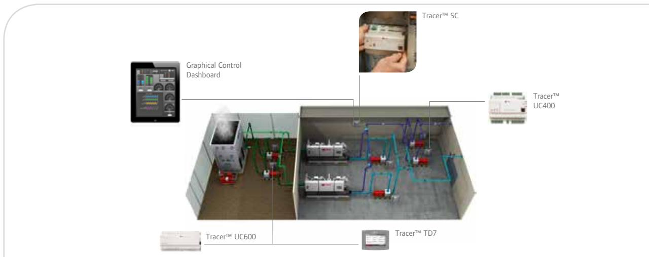
Trane chiller plant controls architecture is built around core high technology components.
