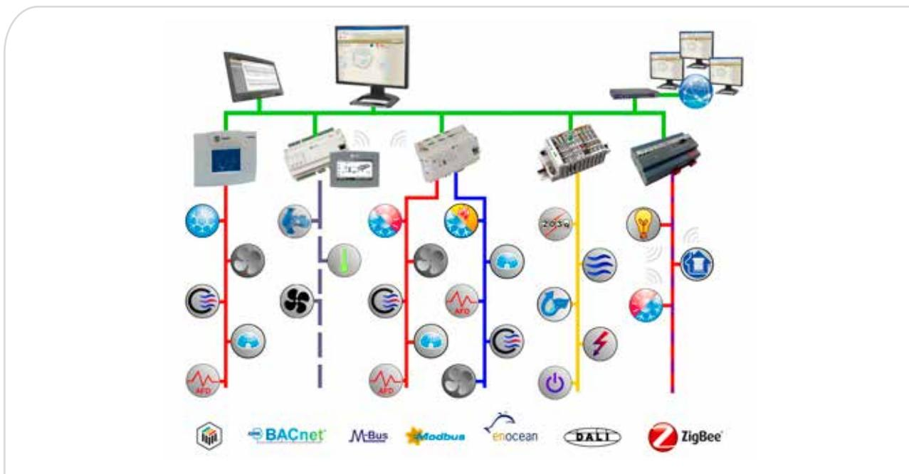
Trane offers an open and secure controls Building Management architecture. The use of native open protocols allows for easy commissioning and facilitates maintenance as well as ensures a scalable and flexible system that can evolve to various controls products. It also allows the integration of third party equipment and BMS systems to the network.
