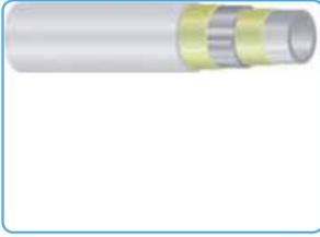
Uponor MLC pipe unites advantages of metal and plastic pipes. The aluminum core acts as an oxygen barrier, reduces heat expansion and gives form-stability for easy and safe installation
