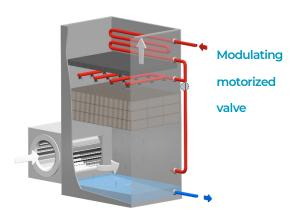
If necessary, the bypass valve is totally closed, the water is first sent to the plume removal battery, and then can be dispersed in its entirety on the runoff surface by distribution nozzles.
