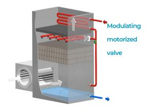
When the dry cooling in not powerful enough part of the water flow goes to the spraying system thanks to the by-pass valve. A temperature probe (option) located in the water outlet send the information to the regulator monitoring the valve. So only the minimum water quantity is sprayed on the packing. This cooling mode lowers the water / air exchange and optimize the power evacuated in the dry coil. According to the ambient conditions, 30 to 70% of the power can be dissipated in dry mode.
