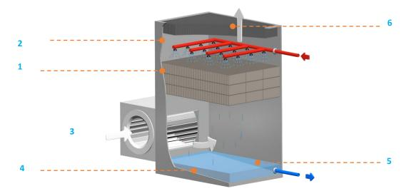
The hot water to be cooled is pumped to the top of the device through pipes. This water is divided and distributed over the heat exchange surface (1) by low pressure water distribution nozzles (2).
