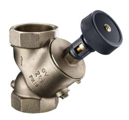
Double regulating valve for static hydronic balancing of pipe networks in closed heating and cooling systems. It offers a measuring function via the valve seat, which is, however, closed with a blind plug when delivered.
