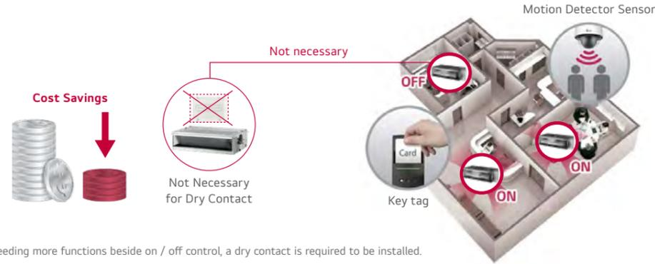
※ In case of needing more functions beside on / off control, a dry contact is required to be installed.
