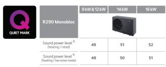
1) Sound power level is measured in accordance with EN 12102-1 and ISO 9614.
